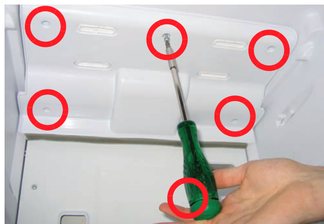
4. Release the 5 screws of the freezer damper housing.
