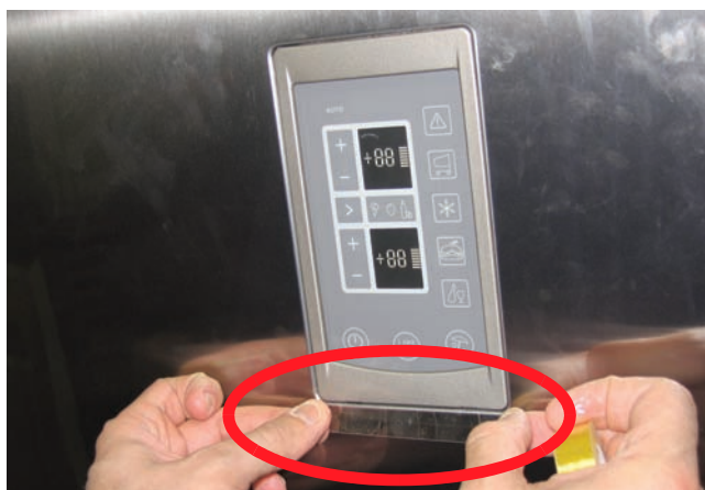
1. Attach some adhesive tape to the bottom of the PCB to prevent damage to the panel.
