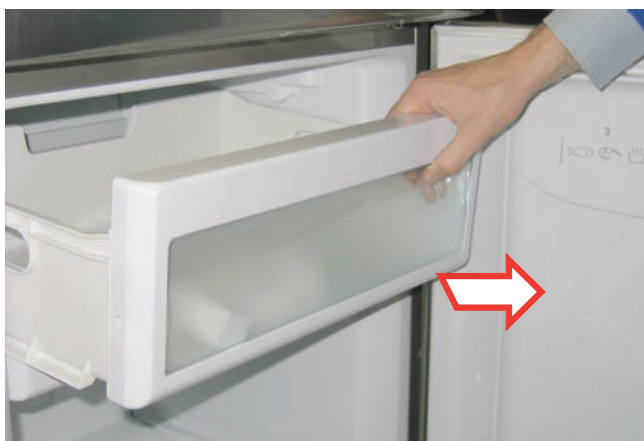
1. Remove the drawers from the freezer compartment.
