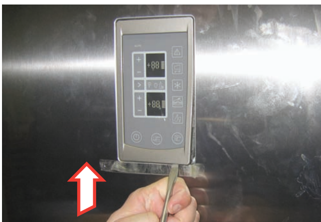
2. Using a screwdriver, prise the PCB off at the bottom on each side.
