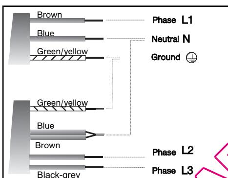
If the unit has a 3 phase 400 V3N connection, and is not working correctly, check that the neutral wire is correctly connected.
